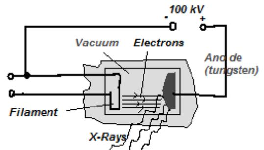
The electrons are produced at the **hot filament**. These electrons are accelerated towards the target metal, which is a high-melting point material such as **tungsten**. The **p.d.** between the **filament** (cathode) and **target metal** (anode) is about **100kV**.
